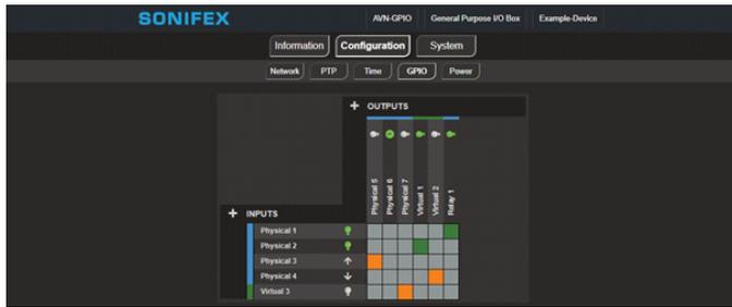
Inputs are shown to the left of the grid and outputs are shown above the grid. Clicking on a box between an input and an output creates a link, allowing an input to drive an output.
