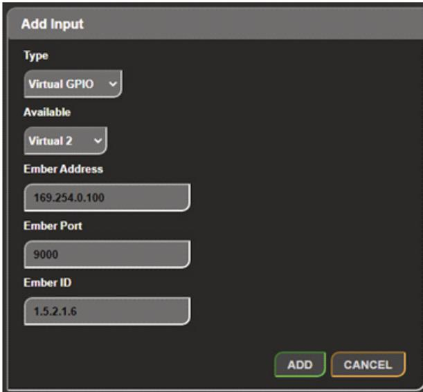
The field 'Ember Address' should be set to the address of the device you would like to connect to. This device must have an Ember provider, for example an AVN-Portal could be used.
