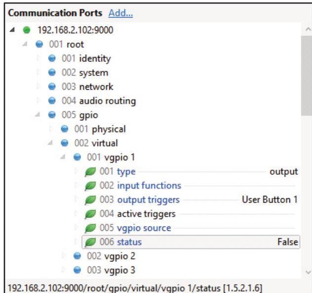
In the example provider tree, the status parameter can be seen, this is a Boolean value that can be added as an input. The raw path to this parameter is 1.5.2.1.6
